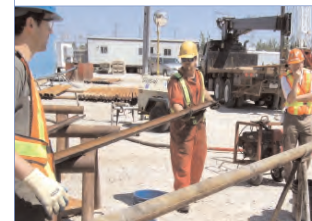
Drill crew displays a 10-foot long section of rock core from DGR2.
